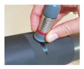
Do *three* measurements on the anilox surface, inside the circle, with the FerroFluid
