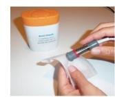
Clean the probe tip with the towel provided in the kit, or with a dry absorbing paper. Do not use alcohol.
