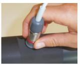
Do *three* measurements on the anilox surface, inside the circle, <u>without FerroFluid</u>
