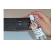
Clean the FerroFluid on the roll surface with the *AniCheck* cleaning fluid
